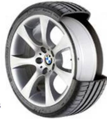
Michelin ZP tyres have reinforced sidewalls which support the vehicle weight in the event of pressure loss. ZP technology is available in the following ranges
